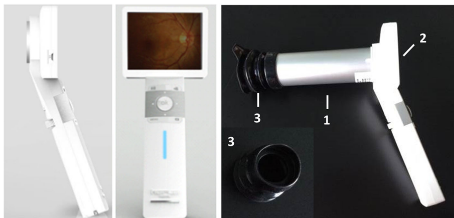
Fig. 1 General diagram of the portable fundus camera prototype. The design is separated into two components: (1) an attachment housing optical components and (2) a liquid crystal display (LCD) monitor with a complementary metal-oxide semiconductor (CMOS) sensor. (3) An eyecup can be fixed with on component 1
