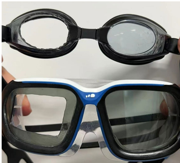
Fig. 1 Eye-socket goggles SG1 (top) and wide vision swimming goggles SG2 (bottom), with the center part of the plastic eye mask for the right eye removed
