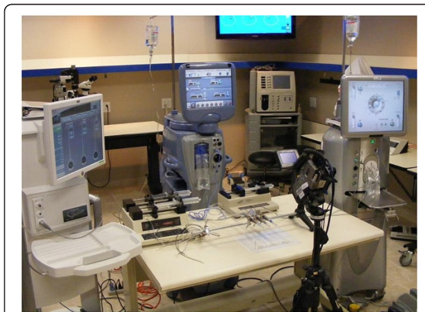
Figure 1 The basic experiment setup. The thermal imaging camera, surrounded by 3 phacoemulsification units.
