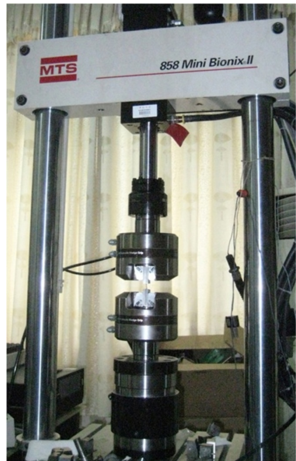
Fig. 3 Biomechanical loading picture of eye material
