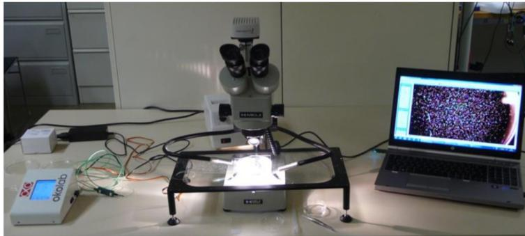
**Fig. 1** Setup for evaluation of glistenings. Left to right: Heated stage used to maintain and monitor the temperature during glistening evaluation; Microscope over a Petri dish including an IOL under test on an illuminated, heated plate; Laptop with image analysis software
