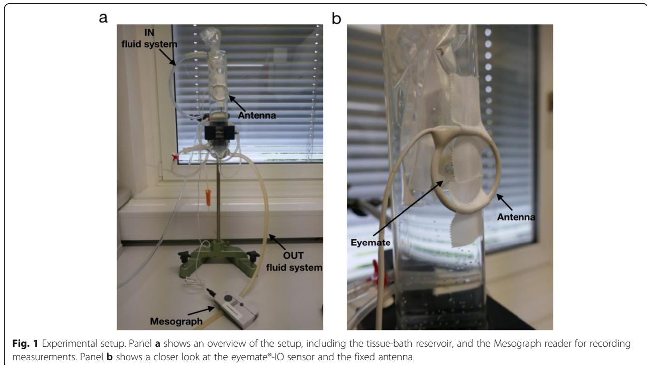
**Fig. 1** Experimental setup. Panel **a** shows an overview of the setup, including the tissue-bath reservoir, and the Mesograph reader for recording measurements. Panel **b** shows a closer look at the eyemate®-IO sensor and the fixed antenna
