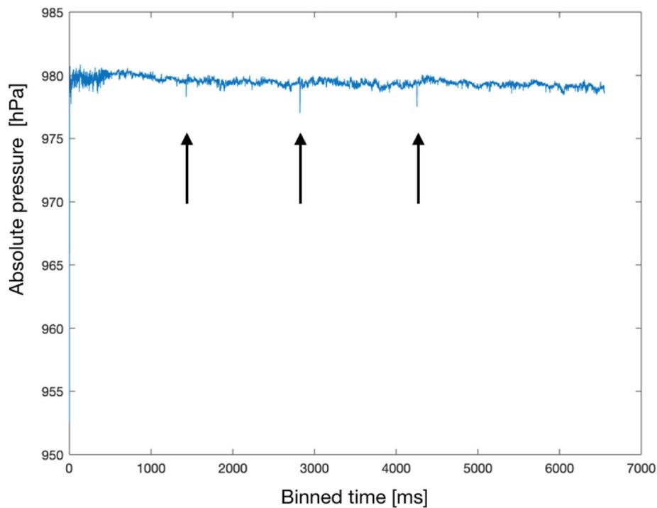
**Fig. 2** “Quasi-continuous” data recorded for a device. We show an example of the data recorded for one of the three tested devices, namely the smartphone. Arrows indicate drop in the signal measurements
