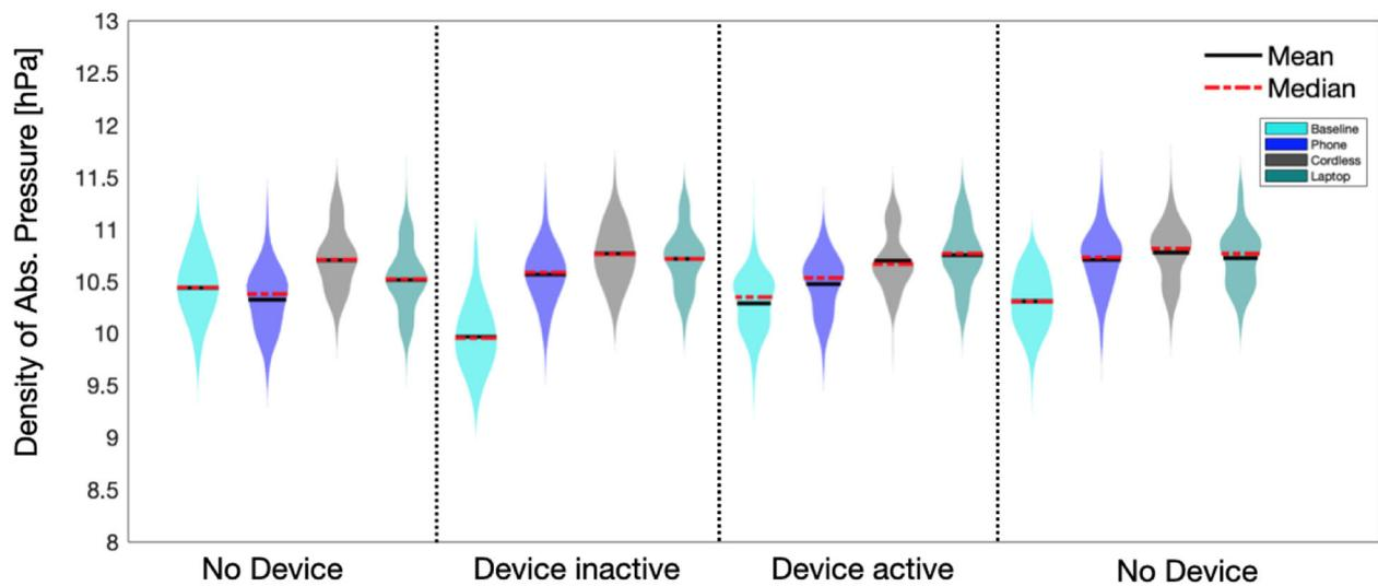
**Fig. 3** Absolute pressure distributions during the four time-events. A kernel density function was applied to the data for plotting purposes. Mean and median of each distribution are indicated with black solid line and red dotted line, respectively
